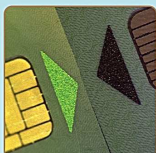
光學變色油墨 Ink with optically variable properties
